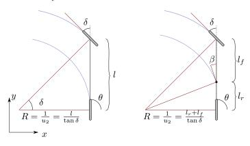
Our vehicle model uses lateral accelleration  $(u_1)$  and curvature of the front-wheel turning  $(u_2)$  as controls. The geometry of the rear-axle centered model (left) can be described as
