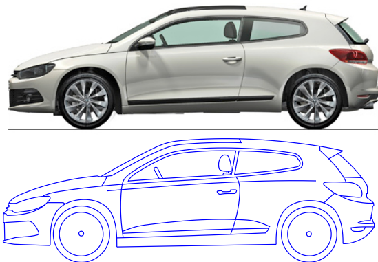
Figure 1: Design curves of a car captured with PCCs.
