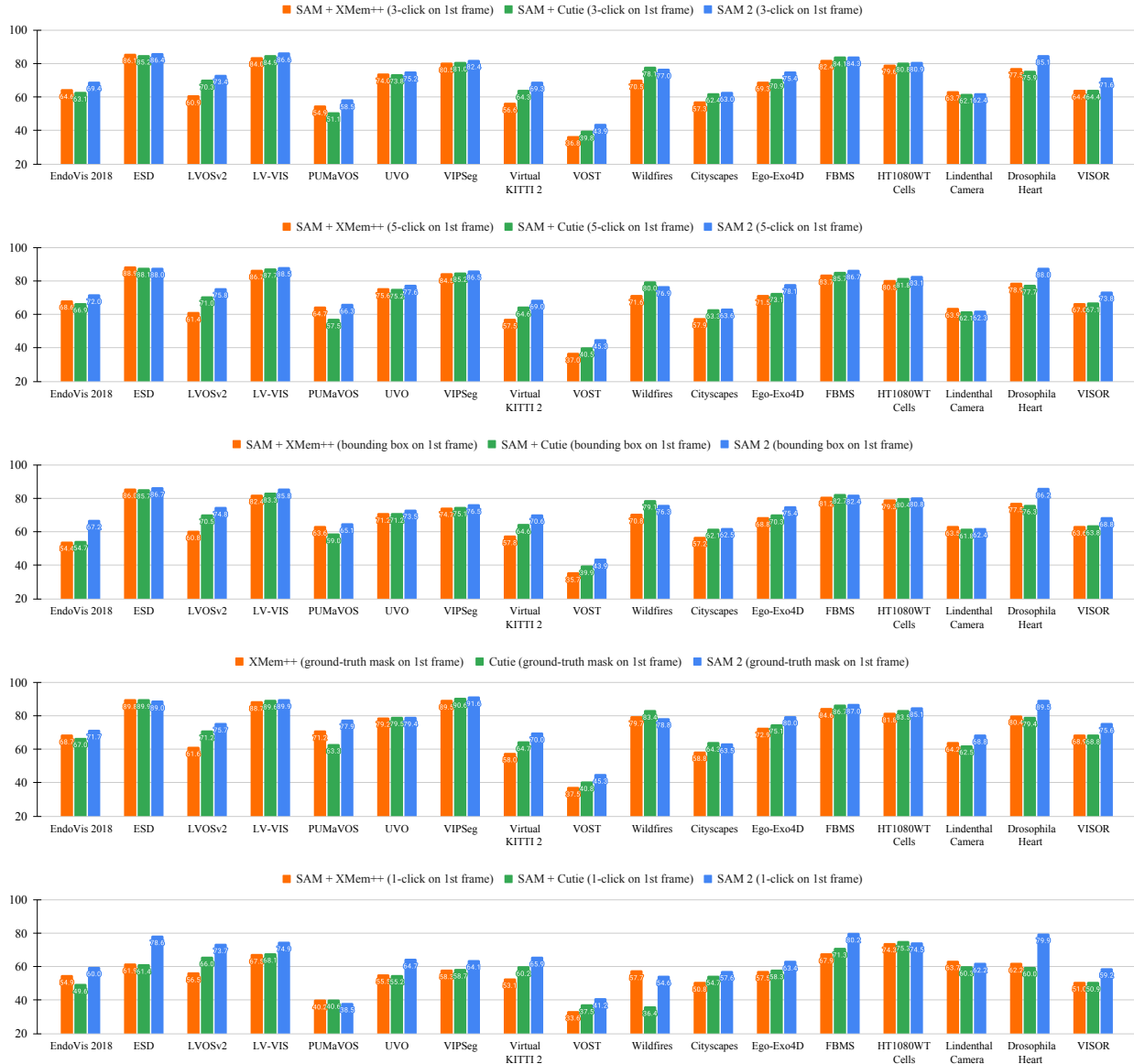
Figure 14 Zero-shot performance on 17 video datasets of SAM 2 vs two baselines (SAM+XMem++ and SAM+Cutie) under semi-supervised VOS evaluation using different prompts (1, 3 or 5 clicks, bounding boxes, or ground-truth masks on the first video frame), with the averaged performance across datasets for each type of prompt shown in Table 4 in the main text. See §E.1.3 for details.
