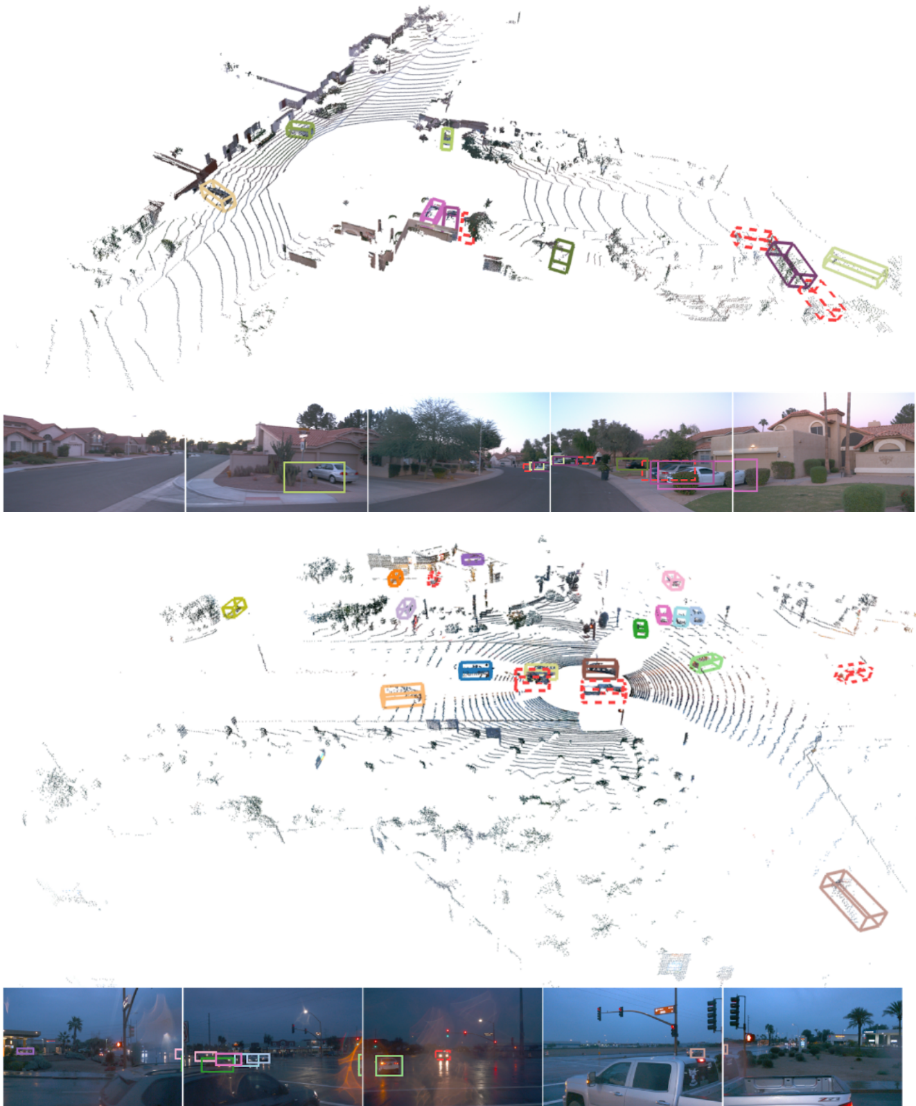
Figure 9. Failure cases examples: In these two challenging cases, the central image (stream) is not sufficient and a vehicle is missed.
