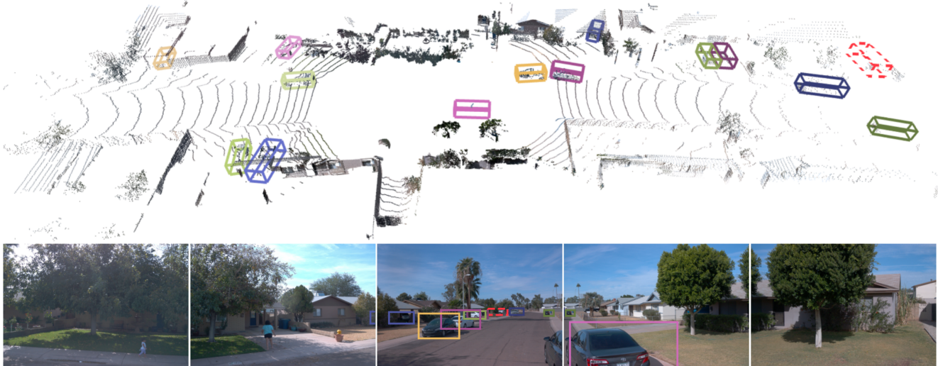
Figure 6. 4D-Net predictions on a scene in the Waymo Open Dataset [47]. Individual instances are shown in different colors. Red boxes indicate errors (dashed lines: FN, solid lines: FP). In this example, all predictions are matching the ground-truth except for a false-negative on the right side (front camera). Note that any misalignments in the camera view are due to projection, not by inaccuracies in the predictions.
