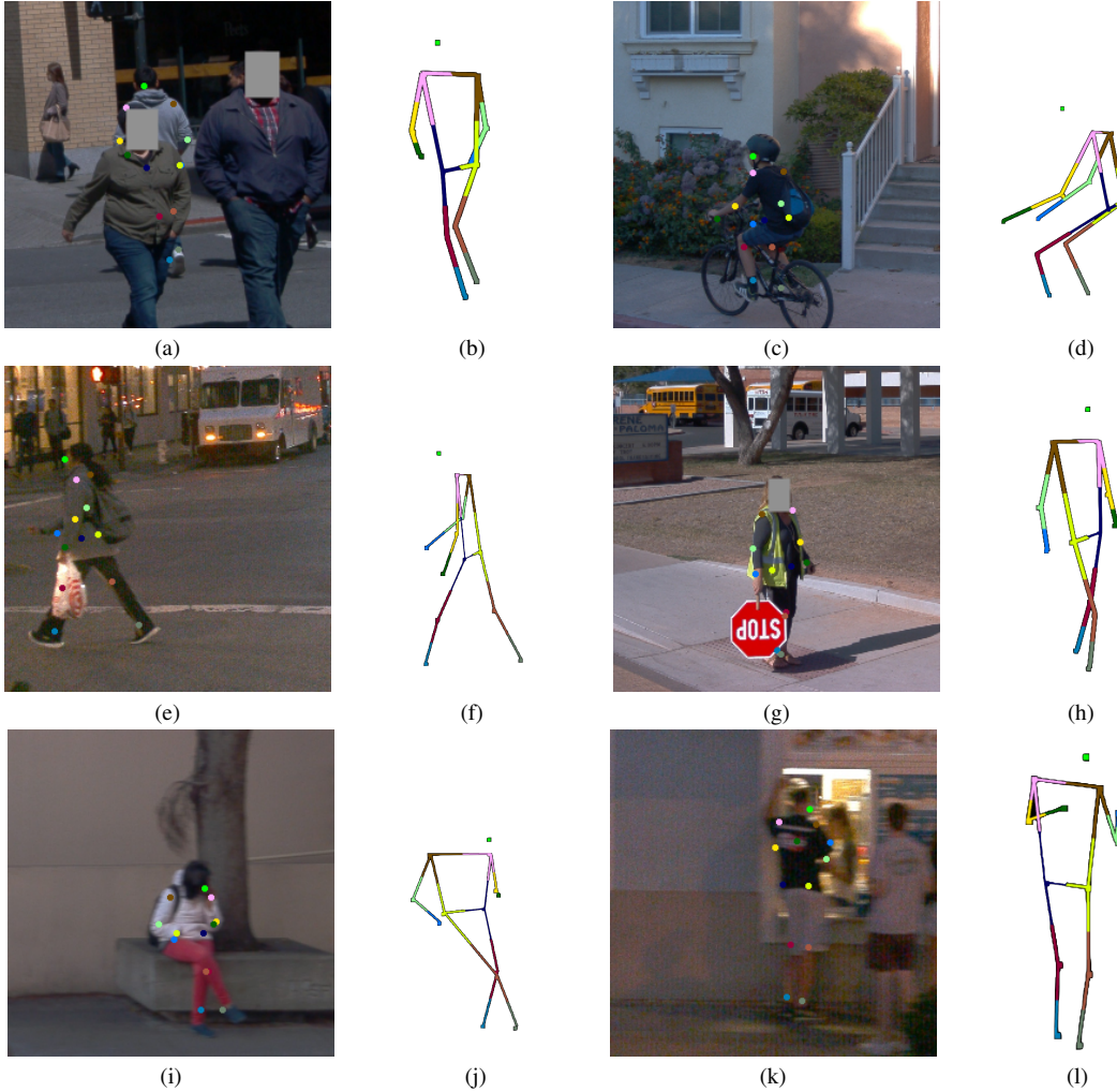
Figure 6. Results on the Waymo Open Dataset. 6b, 6d, 6h, 6l are 3D predictions. 6a, 6c, 6g, 6k show the corresponding 2D projections overlaid on camera images (3D predictions may not be shown under the same viewpoint as the camera images. Best viewed in color). More results can be found in supplementary.
