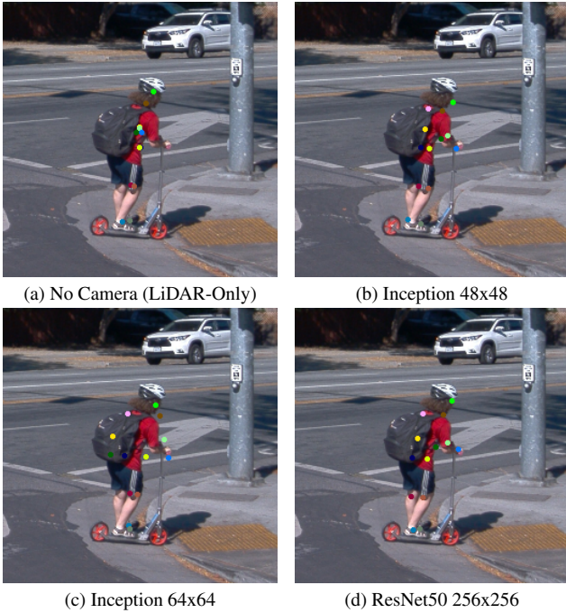
Figure 5. 3D predictions with different camera image sizes and camera network backbones from the Waymo Open Dataset (best viewed in color). ResNet50 with 256x256 image size predicts the most accurate keypoints.
