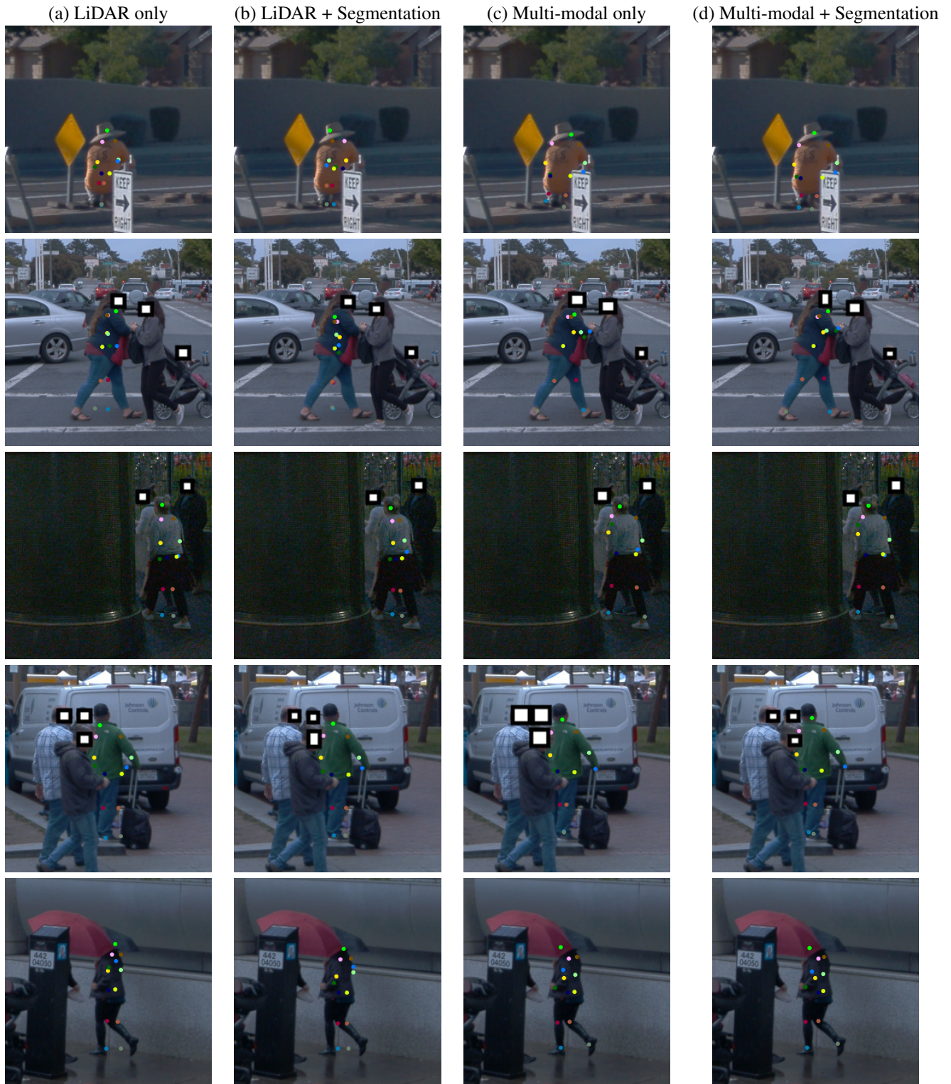
Figure 2. Additional qualitative results on the Waymo Open Dataset, showing the improvement that our approach brings over LiDAR-only model. The columns in each row show: a) LiDAR-only model without segmentation branch; b) LiDAR-only model with segmentation branch; c) multi-modal model without segmentation branch; and d) multi-modal model with segmentation branch. Note that in each case there is either self- or other forms of occlusion that deteriorates LiDAR only results. While segmentation and camera each can provide some additional clue, combining everything produces the best result. Best viewed in color.
