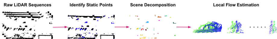
Fig. 2. Proposed NSFP++. Taking as input raw LiDAR sequences (after ground removal), our approach first reasons about the motion status of each point, decomposes the scene into connected components and predicts local flows accurately for each semantically meaningful component.
