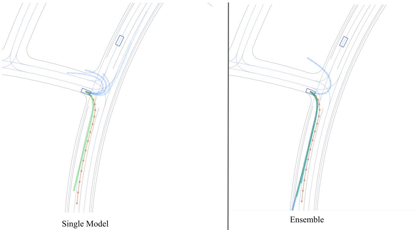
Fig. 14: Here the ensemble correctly predicts that a right turn is much more likely than a u-turn or a left turn from this position.
