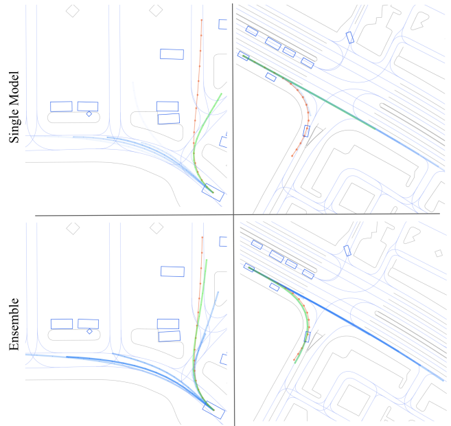
Fig. 6: 2 Qualitative examples for a single teacher models (top row) compared with a K = 28 teacher ensemble (bottom row). Both setups output 6 trajectories after NMS. The red trajectory is the groundtruth, the green is the prediction closest to the groundtruth, and the blue are the remaining predictions. The grid lines represents the background scene including the roadgraph and other agents.
