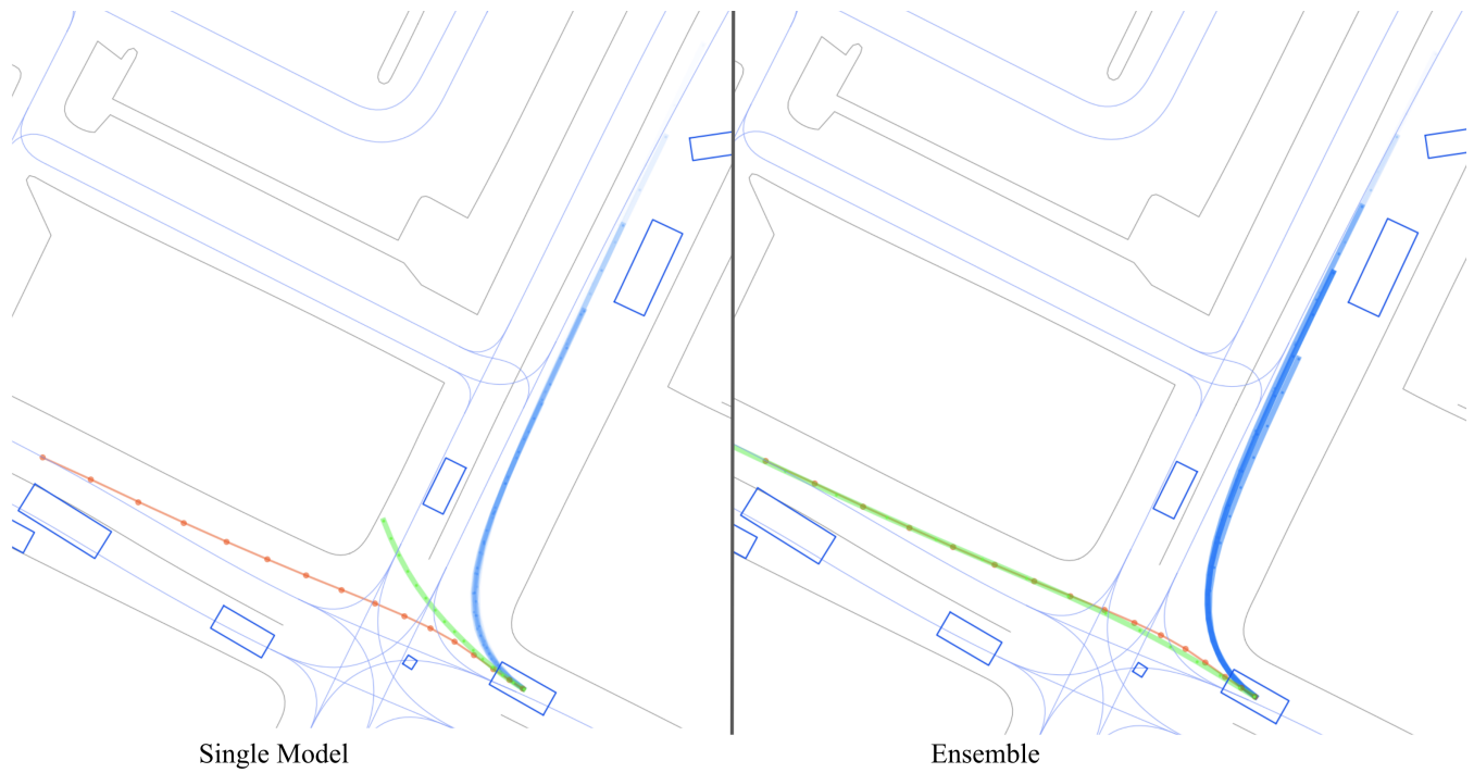
Fig. 9: Here the ensemble correctly predicts a forward trajectory while eliminating the unlikely path that drives off the road predicted by the single model.
