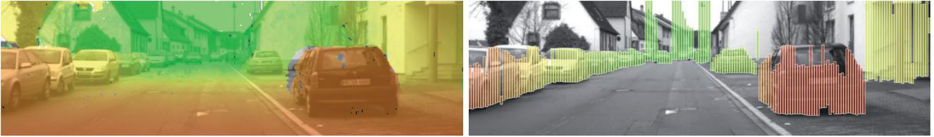
Fig. 2. Low-level SGM disparity image (left) and medium-level Stixel World representation (right) for an urban traffic scene. The colors encode distance from the camera from near (red) to far (green).
