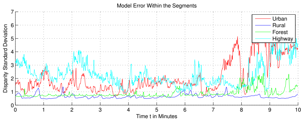
Figure 38: Model error expressed by the average standard deviation of the disparity measurements within the segments. Interestingly, the spikes of the dark blue graph mostly correspond to approaching vehicles within the opposing lane.
