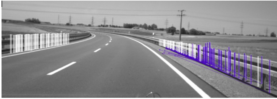
(a) Unreliable optical flow estimates on guard rails lead to wrong Stixel velocity estimates. Additionally, the guard rail is not covered completely.
