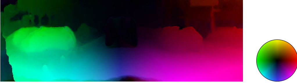
Figure 24: A dense optical flow image for the urban scenario from Figure 12a is shown. The color denotes the direction of the optical flow vectors while the brightness encodes their length. The leading vehicle is almost completely black. This is correct, since it moves at constant distance and therefore does not change its location or scale within the image.
