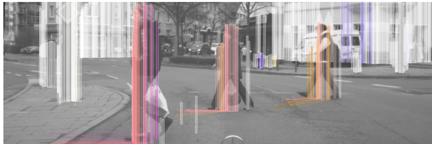
(c) This scenario illustrates the limitation of the Stixel tracking principle with respect to objects that exhibit non-rigid motion, such as pedestrians. The centers of the bodies are tracked quite well, however, the legs and feet are not. For this purpose, a more detailed motion model for pedestrians would be required. For instance, point-based tracking, such as scene flow or 6D-Vision, or schemes that explicitly rely on the shape of human bodies would help to track pedestrians more reliably.
