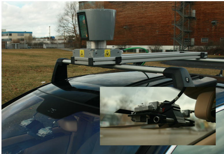
Figure 30: Photograph of the used test vehicle. It shows the installation of the stereo camera system behind the windshield and the Velodyne LIDAR HDL-64E S2 mounted to the roof rack. This LIDAR unit is used for benchmarking the measurement accuracy that is achieved by using Stixels.
