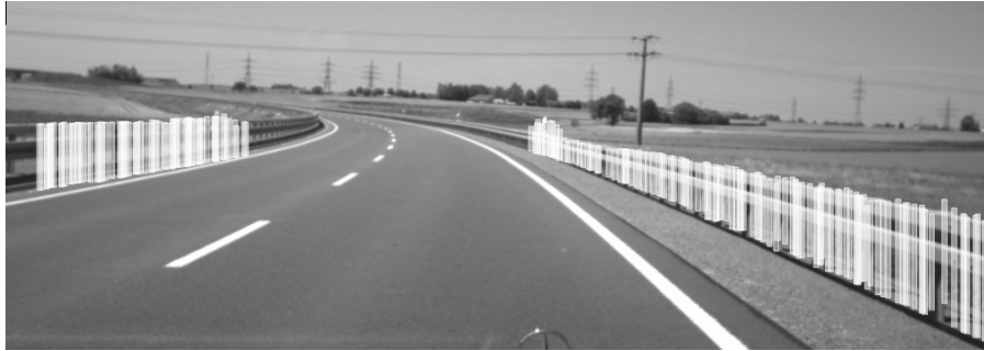
(b) In contrast, successful optical flow computation allows to obtain correct Stixel velocity estimates. The rails is covered much better.
