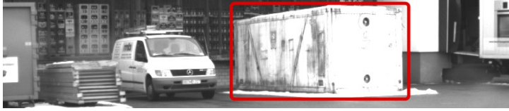
Figure 33: For the evaluation the container right to the parked car was used (red box). That object is well-textured, exhibits no protruding parts and satisfies the Stixel object model constraints almost perfectly.
