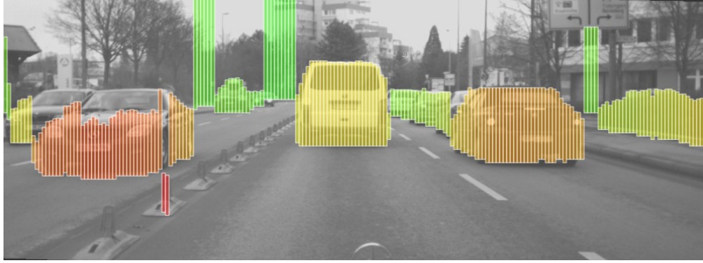
Figure 2: The Stixel World as initially published in [9]. Every Stixel represents a certain part of the first obstacle to encounter along that particular viewing direction. The Stixel coloring encodes the distance to the object. Red means close and green is far away. Stixel boundaries are marked white.
