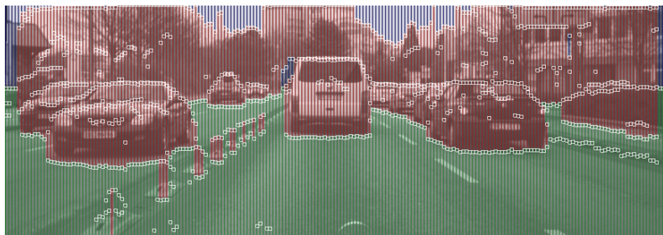
Figure 19: This illustrations shows the labeling result for the urban scenario from Figure 12a. Using ground level estimation, the approach is capable to detect and segment even slight elevations of the ground surface. This can exemplarily be seen on the right side of the image with the sidewalk.
