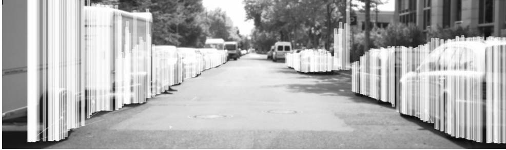
(a) Correct estimation of the environment to consist of static objects only. Thus, all Stixels are drawn with a white coloring which denotes a velocity close to zero.
