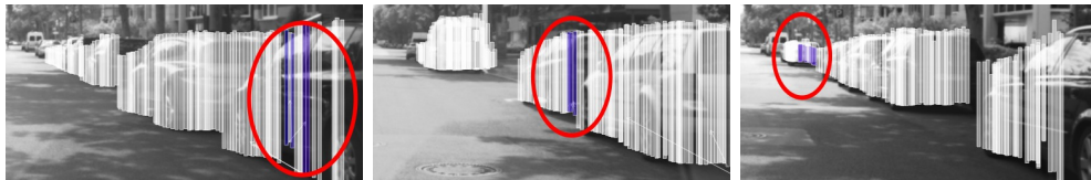
(b) Three typical sources for velocity errors during tracking within static environments are illustrated. The left figure shows a reflecting surface, the middle figure shows a jump in depth, and the third figure shows difficulties with motion estimation at large distances.
