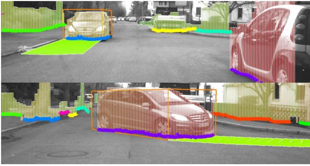
Fig. 9: Application of Stixels in a vehicle tracking system. The color bands at the bottom mark groups of Stixels, the boxes around the cars show their estimate orientation and the green “carpet” illustrates the predicted trajectory of the vehicle.
