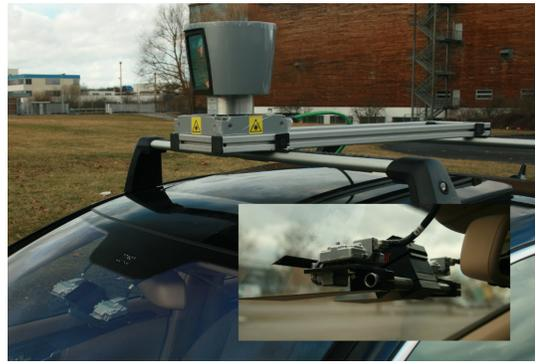
Fig. 10: Photograph of our test vehicle showing the installed stereo camera system behind the windshield and the Velodyne *LIDAR HDL-64E* mounted to the roof rack.
