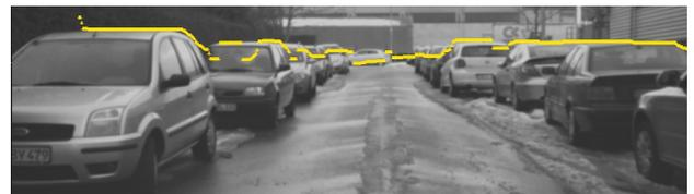
Fig. 8: Result of the height segmentation after applying DP. The red line indicates the segmentation of foreground and background.
