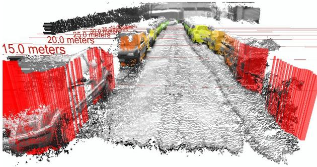
Fig. 2: Visualization of the triangulated SGM data and the 3D Stixel representation.
