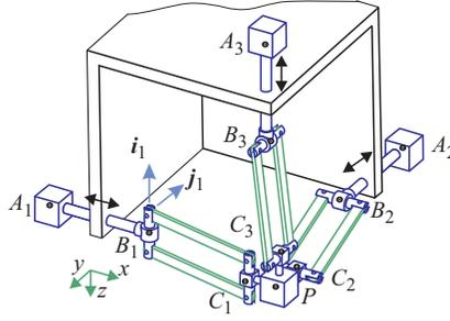
Figure 1. Orthoglide kinematic architecture
