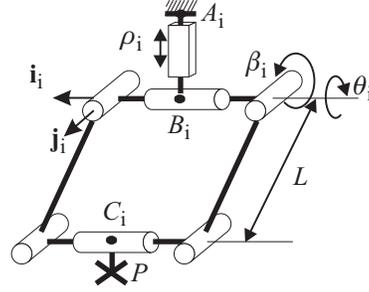
Figure 2. Leg kinematics
