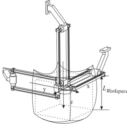
Figure 4. Cartesian workspace and isotropic configuration of the Orthoglide mechanism
