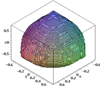
Figure 3. Dextrous workspace of the Orthoglide mechanism
