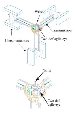
Figure 14: Six-dof haptic device 3T+2R+1R
