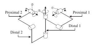
Figure 10: The hybrid agile eye with two-dof in serial with a revolute actuated joint ③
