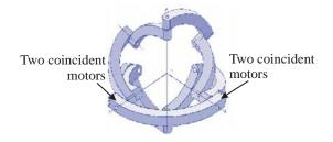
Figure 9: Redundant spherical wrist
