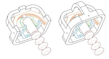
Figure 16: New design of the wrist
