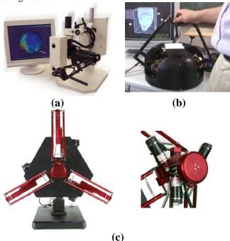
Figure 3: Three haptic devices with six-dof with (a) serial architecture, (b) parallel architecture and (c) hybrid architecture
