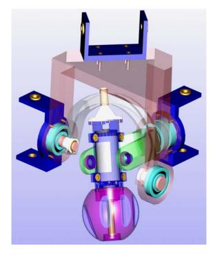
Figure 17: CAD model of the new wrist
