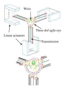
Figure 13: A six-dof haptic device 3T+3R
