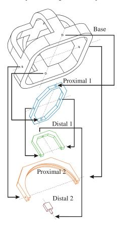
Figure 15: New part design of the agile eye
