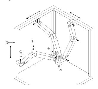
Figure 5: A fully isotropic parallel mechanism
