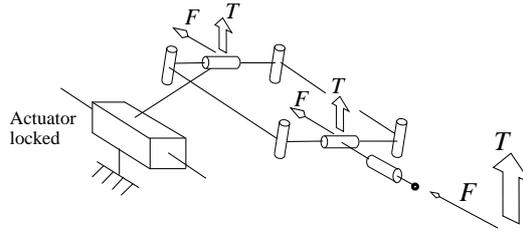
FIG. 4 – Forces transmitted in a leg
