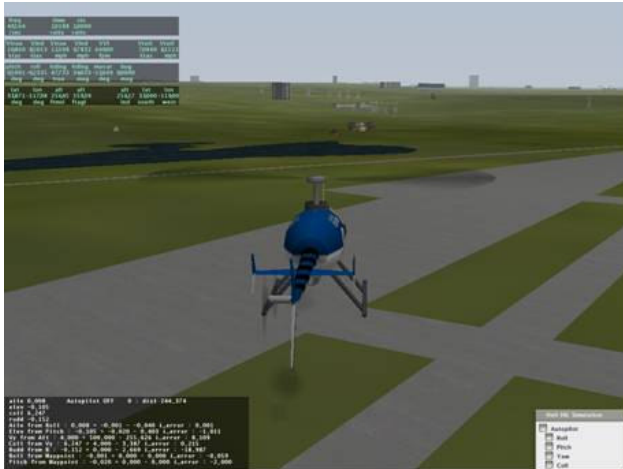
Figure 6: PID controller hovering RC-02 in X-Plane
