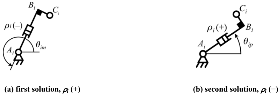
Figure 3. The two inverse kinematic solutions of the i^{\text{th}} leg of the robot.
