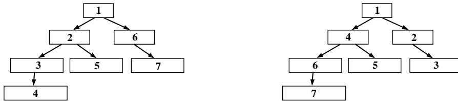
Fig. 11. In the distributed deployment algorithm of Table VI, explorer agents search the partition tree \mathcal{T}_{\mathcal{P}} depth-first for leader or proxy tasks they could perform. An agent in a cell, say c_{\xi} , can always order the gap edges of c_{\xi} , e.g., counterclockwise from the parent gap edge. The depth-first search progresses by the explorer agent always moving to the next unvisited child or unexplored gap edge in that ordering. The agent thus moves from cell to cell deeper and deeper until a leaf (a vertex with no children) is found. Once at a leaf, the agent backtracks to the most recent vertex with unvisited child or unexplored gap edges and the process continues. As an example, (left) integers (not to be confused with PTVUIDs) shows the depth-first order an agent would visit the vertices of \mathcal{T}_{\mathcal{P}} in Fig. 3f if the gap edges in each cell were ordered counterclockwise from the parent gap edge. If the agent instead uses a gap edge ordering cyclically shifted by one, then (right) shows the different resulting depth-first order. If each agent uses a different gap edge ordering, e.g., cyclically shifted by their UID, then different branches of \mathcal{T}_{\mathcal{P}} are explored in parallel and the deployment tends to cover the environment more quickly. Cf. Fig. 10.
