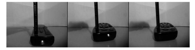
(A simple example of how a robots vision may be augmented. The two images on the left represent the fact that cameras are Infra-Red sensitive, however infra-red light lies outside the scope of the vision of Human beings, and as a result what a human being may see is depicted by the image on the right)
