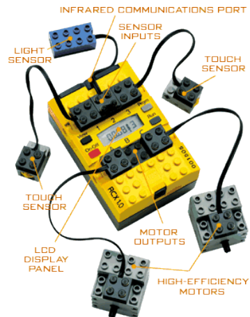
Figure I-B-1: RCX 2.0 Linked to different sensors and actuators.
