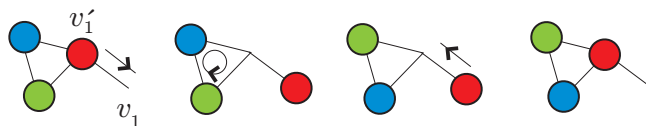
Fig. 9. With one empty vertex, pebbles on a triangle can be arranged to achieve any desired configuration. This generalizes to an arbitrary TECC.
