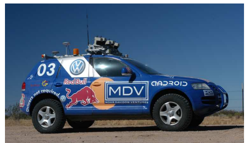
Figure 1: Stanley won the 2005 DARPA Grand Challenge by completing a 132 mile desert route in just under 7 hours. Data from this race is used to evaluate the terrain perception method described in this paper.
