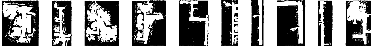
Figure 6: Partial maps used for evaluation of map merging. The maps were taken from three different environments. In each experiment, one robot built such a partial map and receives data from another robot collected in the same environment. The robot has to determine when and if so where the other robot is in its partial map.
