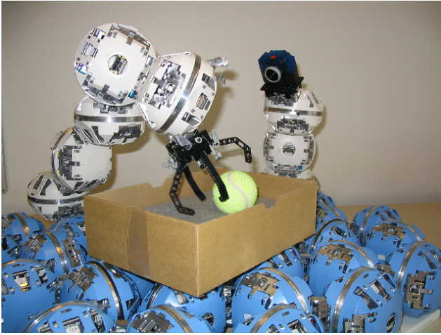
Fig. 1. Arms and conveyor belt constructed of ATRON modules [6]
