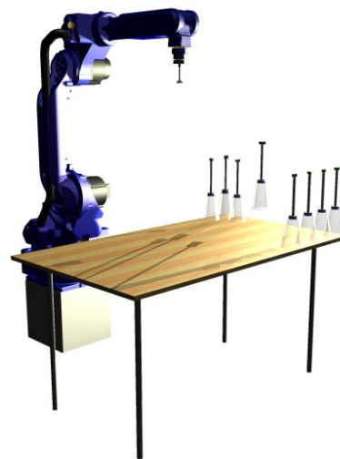
Fig. 3. CAD assembly model of the robotic material handling cell. A robot program will be generated from this model.
