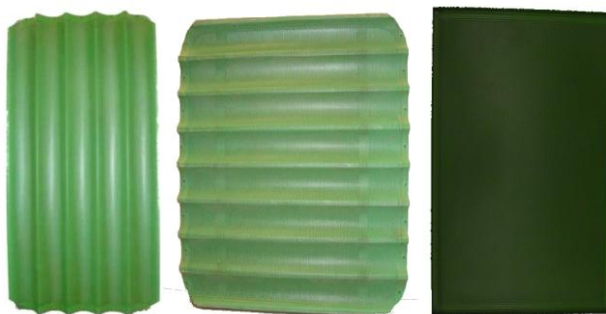
Fig. 5 Three different workpieces produced by FLUPOL. Horizontal wavy-surface plate (left), vertical wavy-surface plate (middle) and smooth surface (right)
