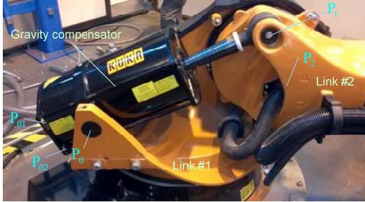
Fig. 1. Gravity compensator of robot KUKA KR-270 TM
