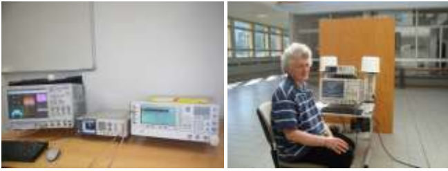
Figure 3. Experimental setup: UWB acquisition system (left) and one of the measurement configurations (right)
