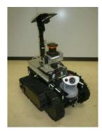
Fig. 1. The surveyor type robot which has a 3D laser scanner.
