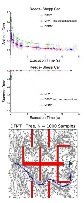
Fig. 1. Top: Simulation results for the Reeds-Shepp car system with a maze obstacle set. The error bars in each axis represent plus and minus one standard error of the mean for a fixed sample size n. Bottom: Example DFMT\* tree for n=1000. The feasible path returned is highlighted in blue with car direction at each sample state denoted by an arrow.
