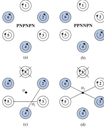
Fig. 3. (a) Standard rotor arrangement, (b) new rotor arrangement, (c) the 1-st rotor of the PNP system fails, (d) the 1-st rotor of the PPNN system fails.
