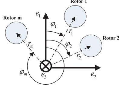
Fig. 2. Geometry definition for multirotor system
