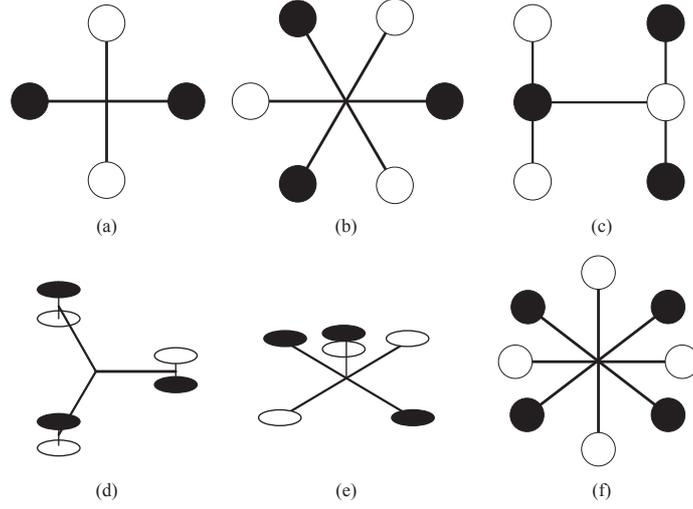
Fig. 1. Different configurations of multirotor helicopters (the white disc denotes that the rotor rotates clockwise and the black disc denotes that the rotor rotates anticlockwise)
