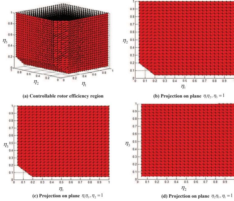
Fig. 4. Controllable region of different rotors' efficiency parameter for the PNPNP hexacopter
