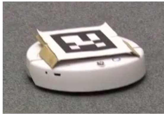
Figure 1: Roomba fitted with GPS tag
