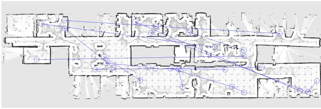
(a) Tasks of the robots and the roadmap used for planning.
