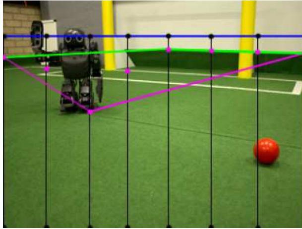
Figure 3: Camera frame and green horizon detection results: The image is a real frame captured by the DARwIn-OP onboard camera of the playing field. It shows several important features - ball, goalposts, another robot and several field lines. Notice that all those features can still be detected if we consider only the part of the image below the so-called green horizon; i.e. , the point where the field ends. The blue line indicates the true horizon, obtained from kinematics information about the robot’s head angle. The vertical lines are scanlines used to determine where the green pixels start (marked by the magenta markers). Finally, the green horizon is calculated as the top segments of the convex hull associated to those markers.
