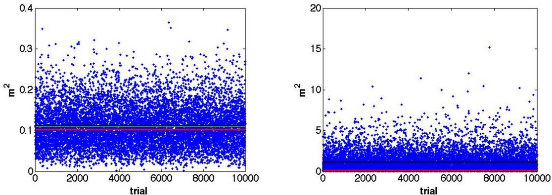
Figure 4: Varying ratio between linear and angular speed. Values of  $D(1)^2$  for  $10^4$  trials together with the value of  $D(1)^2$  for the trajectory without noise (red line), the value of  $\langle D(1)^2 \rangle$  obtained by averaging  $D(1)^2$  on the trials (green line) and the value of  $\langle D(1)^2 \rangle$  obtained by our formulas (black line).  $K_\theta = K_r = 0.01m$  and  $K_\theta = K_r = 1m$  in the left and right image, respectively.
