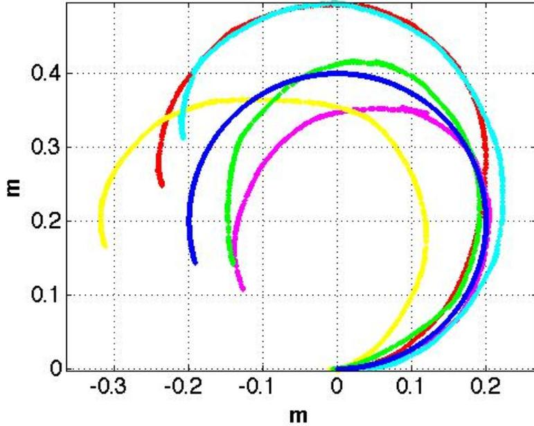
Figure 1: Trajectories generated in the case of constant ratio between linear and angular speed. The blue line is the trajectory generated without noise (i.e.,  $K_\theta = K_r = 0$ ) and the other lines are five trajectories obtained by setting  $K_\theta = K_r = 0.01m$ .
