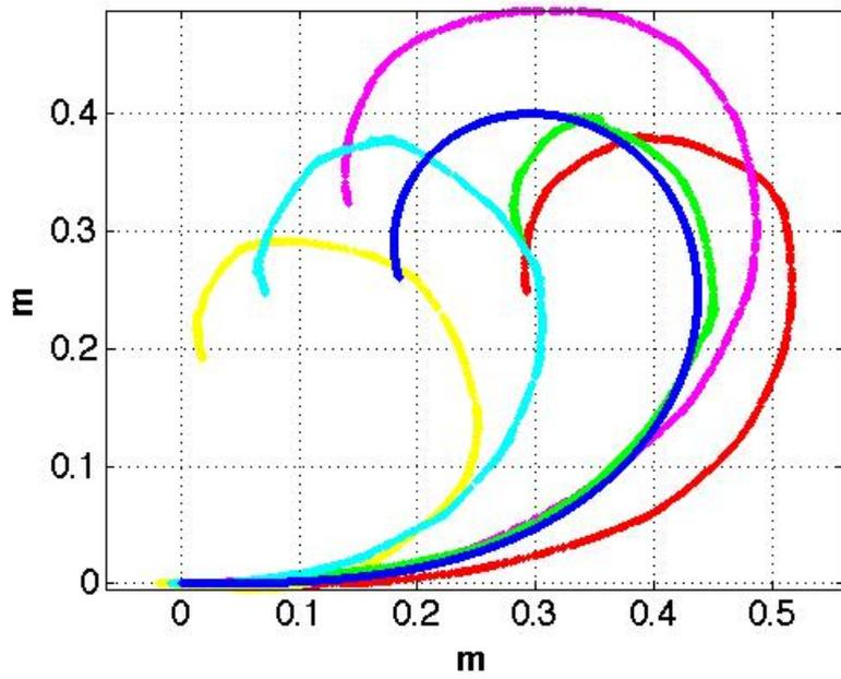
Figure 3: Trajectories generated in the case of varying ratio between linear and angular speed. The blue line is the trajectory generated without noise (i.e,  $K_\theta = K_r = 0$ ) and the other lines are five trajectories obtained by setting  $K_\theta = K_r = 0.01m$ .
