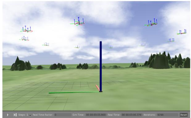
Figure 5: Holding pattern in the CRATES simulator. Ten units coordinate their flight in a circular formation. In this example,  $N = 10^4$  samples, control noise is  $\sigma_u^2 = 0.1$  and horizon  $H = 1$  sec. Cost parameters are  $v_{\min} = 1$ ,  $v_{\max} = 3$ ,  $C_{\text{hit}} = 20$  and  $d = 7$ . Environmental noise and sensing uncertainties are modeled using realistic parameter values.
