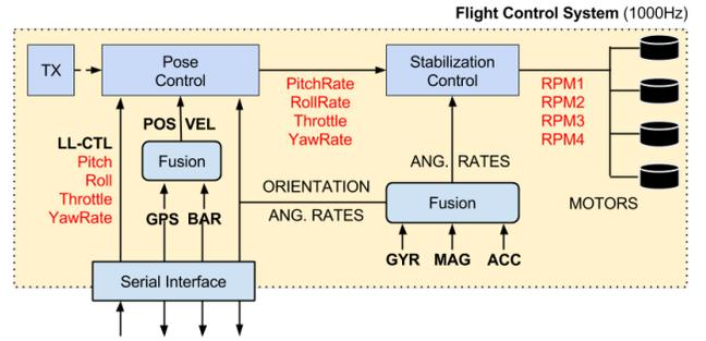
Figure 2: The flight control system (FCS) is comprised of two control loops: one for stabilization and the other for pose control. A low-level controller interacts with the FCS over a serial interface to stream measurements and issue control.
