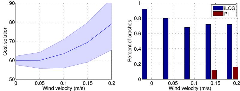
Figure 4: Results: **Drunken Quadrotor with wind**: For different wind velocities and fixed control noise  $\sigma_u^2 = 0.5$ . (Left) cost of the obtained solutions and (Right) percentage of crashes using iLQG and PI.
