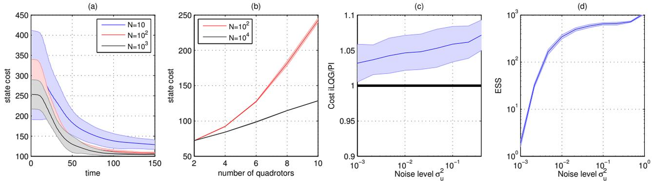
Figure 6: **Holding pattern:** (a) evolution of the state cost for different number of samples  $N = 10, 10^2, 10^3$ . (b) scaling of the method with the number of agents. For different control noise levels, (c) comparison between iLQG and PI control (ratios  $> 1$  indicate better performance of PI over iLQG) and (d) Effective Sample Sizes. Errors bars correspond to ten different random realizations.
