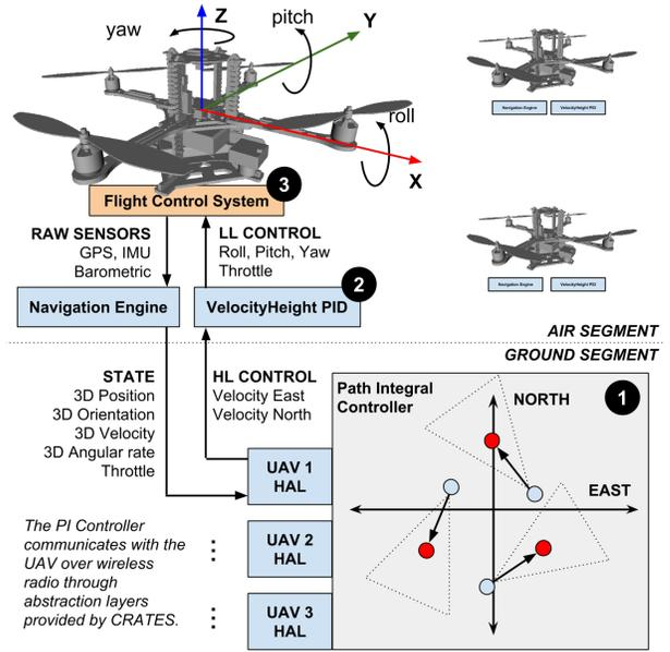
Figure 1: **Control hierarchy:** The path-integral controller (1) calculates target velocities/heights for each quadrotor. These are converted to roll, pitch, throttle and yaw rates by a platform-specific Velocity Height PID controller (2). This control is in turn passed to the platform’s flight control system (3), and converted to relative motor speed changes.
