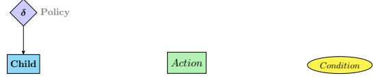
(a) Decorator node. The label describes the user defined policy. (b) Action node. The label describes the action performed. (c) Condition node. The label describes the condition verified.
