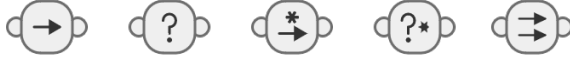
Fig. 2. The visual representation of the core node types. From left to right: Sequence, Priority, MemSequence, MemPriority, Parallel
