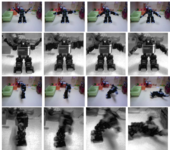
Fig. 4. Sample images from our Robot database for two activities (arms moving and falling) and their normalized images. Four sample images per activity. (Best viewed in color)
