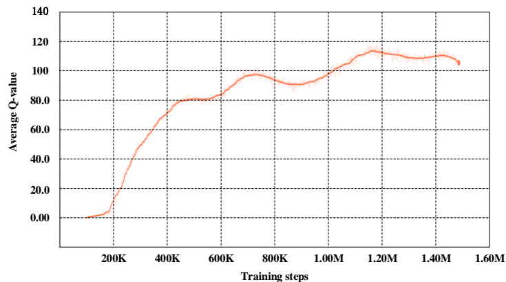
Figure 5: Average Q-value during the training process. After 13 hours, the average value reaches 110, we then used the policy network for autonomous driving without vehicles around.
