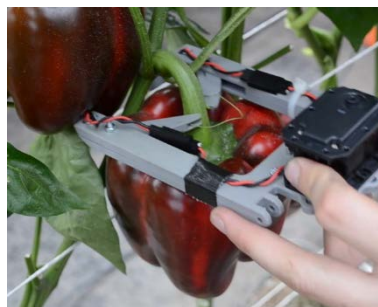
(e) wire cutter prototype – before attachment
