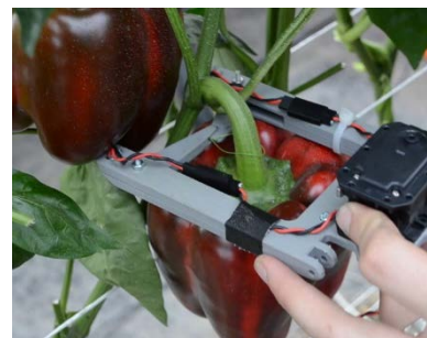
(f) wire cutter prototype – after attachment
