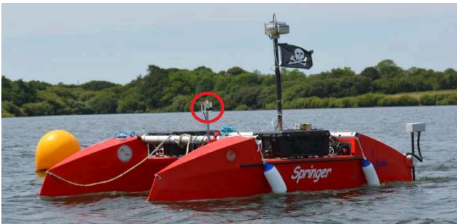
Fig. 3: The unmanned surface vehicle. The camera (circled in red) is mounted on the left hull, pointing sideways.
