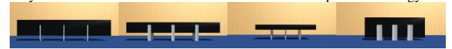
Fig. 2: Four parameterizations of the same Hexapod model. Though not visualized here, masses, moments of inertia, densities, and centers of mass of the links also are parameterized. More complex robots can have larger design spaces.
