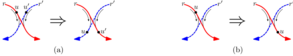
Figure 6 – Transition of the position of the robots (represented by solid points) in the neighborhood of a communication link. (a) Two robots u and u' arrive at a communication link at the same time, then they keep their trajectories. (b) Robot u arrives at the link position and there is no robot in the neighboring trajectory, then u shifts to the neighboring trajectory.
