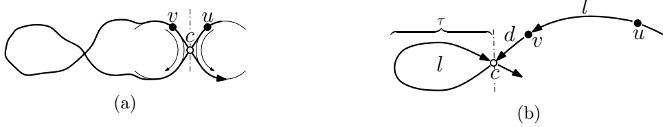
Figure 9 – (a) The length of the tie to the left of the dash-dotted vertical line is equal to the length of the section of ring from u to v . (b) The robots u and v prevent each other from starving because the distance between them is equal to the length of a tie in the same ring.
