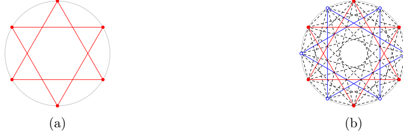
Figure 11 – (a) Circulant graph C_6\{2\} . (b) Circulant graph C_{12}\{1, 3, 4, 5\} which is the K_{6,6} -augmentation of C_6\{2\} , with solid points denoting the nodes of the original graph, and non-solid ones, the vertices of its clone. Original and cloned vertices are connected with dashed edges.
