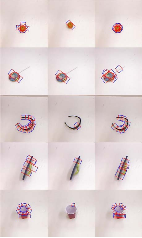
Fig. 4. Detection results in Cornell Grasp Dataset. The first column is ground-truth oriented rectangles. The second column is the visualization of Top1 grasp detection result. The third column is the results of multi grasps.
