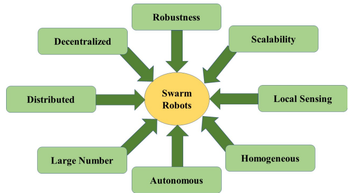
Fig. 6: Characteristics of the cooperative or swarm robots. Distribution, decentralization and robustness are the main features that make them different form single robotic system.
