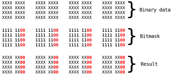
Fig. 1: Bit masking operation, here with 8 bits integer and 2 bits masked. Note the recurrent patterns of zeros in the resulting sequence
